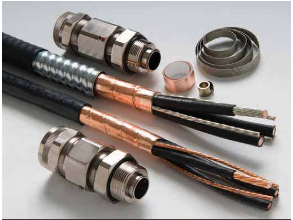
Metal covering of galvanized steel interlocking metal armor acts as a backup low impedance path.
